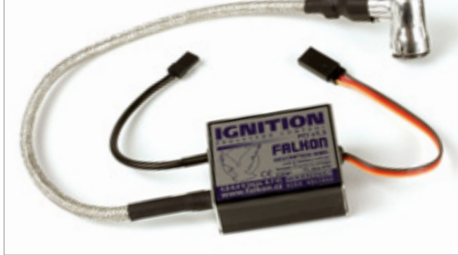
The Falcon electronic ignition system comes with the engine. Notice the shielded spark-plug cable and cap.
