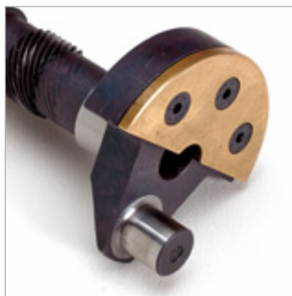
The crankshaft has a brass counterweight plate screwed onto it. The ignition-timing magnet is in the crankpin.
