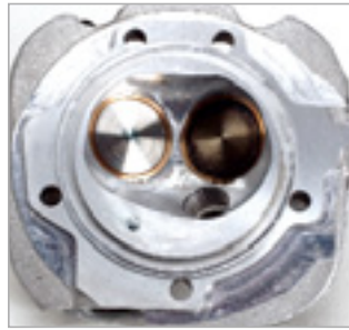
Two substantial valves dominate the hemi-shaped compression chamber.
